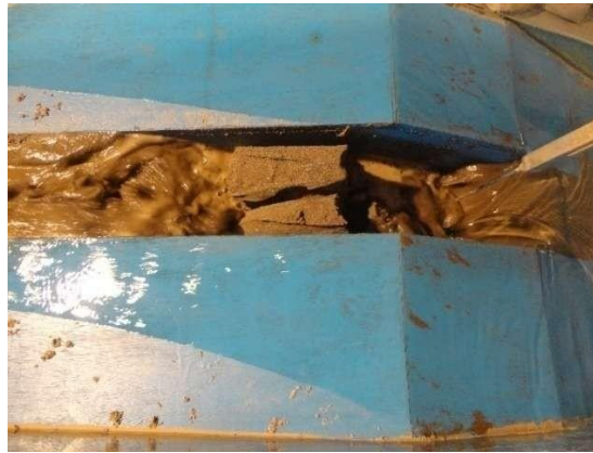
Figure 6 (b): Caveing in of sediment
