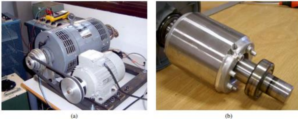
Fig. 9. (a) Experimental setup for 1.1 kW motors tests. (b) Bar breakages in the induction motor rotor. Table 1 Frequency bands for the high-level wavelet signals.
