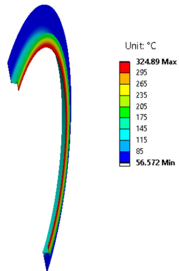
Figure 22. Temperature distribution at kiln hood
