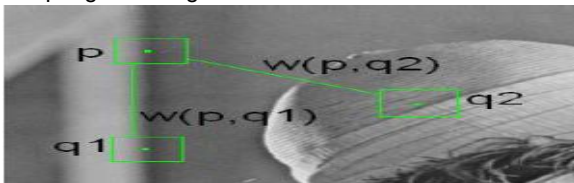
Fig1.3: Example of self-similarity in an image. Pixel sp and ql have similar neighbourhoods, but pixel sp and q2 do not have similar neighbourhoods. Because of this, pixel ql will have a storage influence on the denoised value of p and q2.
