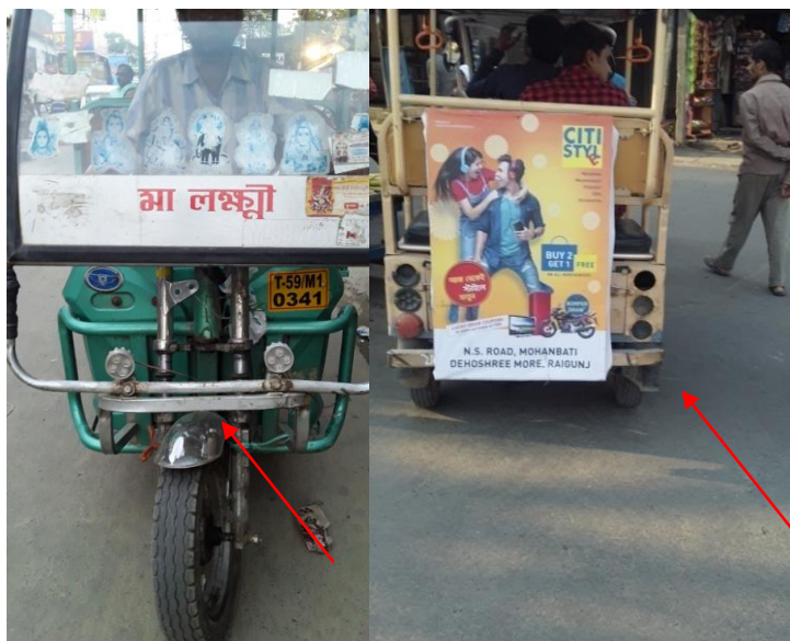
Plate.20: Headlight and backlight is poor condition in Toto
