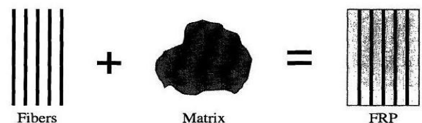
Fig. 1: Formation of Fiber Reinforced Polymer Composite
