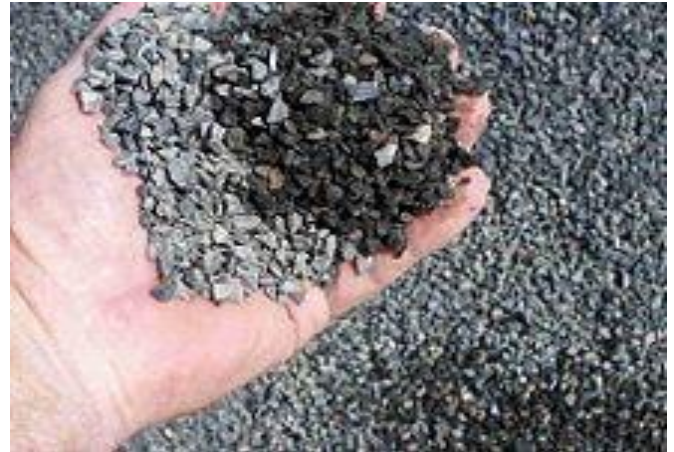
Figure 2: 10 mm Graded Crushed Aggregates.
