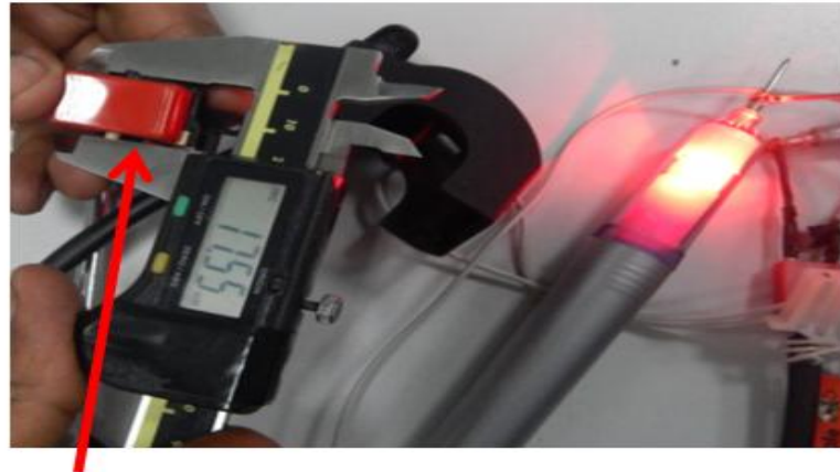
Figure 7: No flickering / continuity missing observed when base pressed by 0.51 mm from base pivot side.
