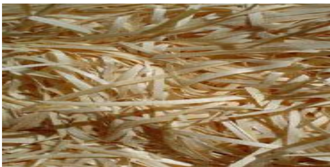
Fig V: Wood Wool Cooling Pad
