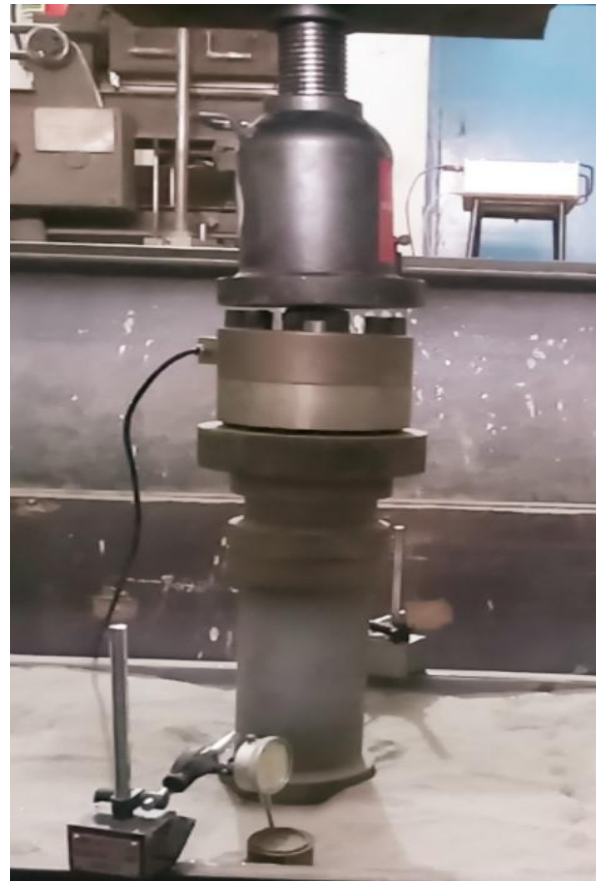
Fig. 5 Model plate load test being done.
