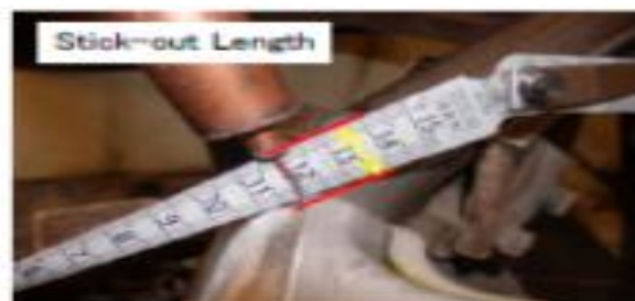
Figure.10: welding wire setting for problem 3.
