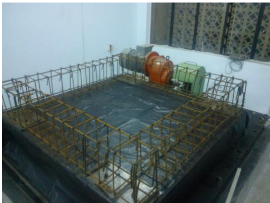
Figure 3 Foundation on Shake Table
