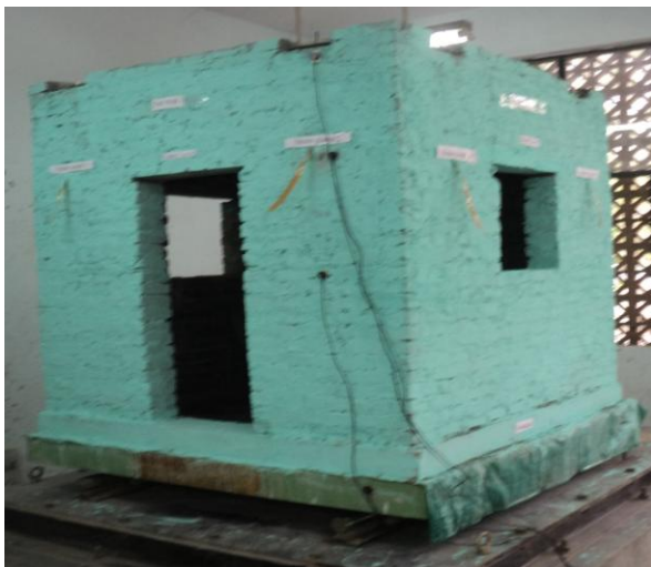
Figure 5 Model on Shake Table Before Test
