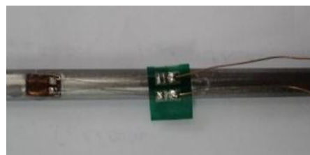
Figure 1 Strain gauge pasted on bar
