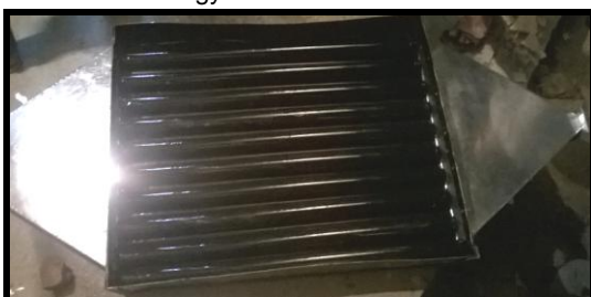
Thermal energy storage system, aluminium tubes colored with black paint.
