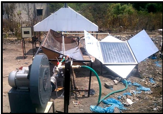
Figure: Overall view of solar dryer (Sunshine)
