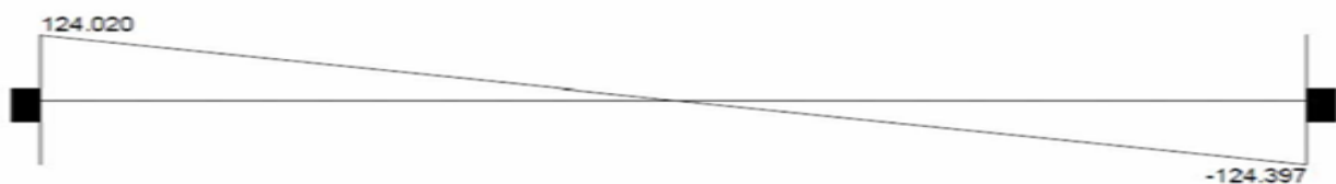
Fig- 4: SFD for beam 226 for 40 % release in STAAD.Pro V8i
