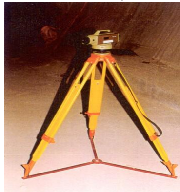
Fig 1.3: Pictorial view of N3 precision level for deflection measurement
