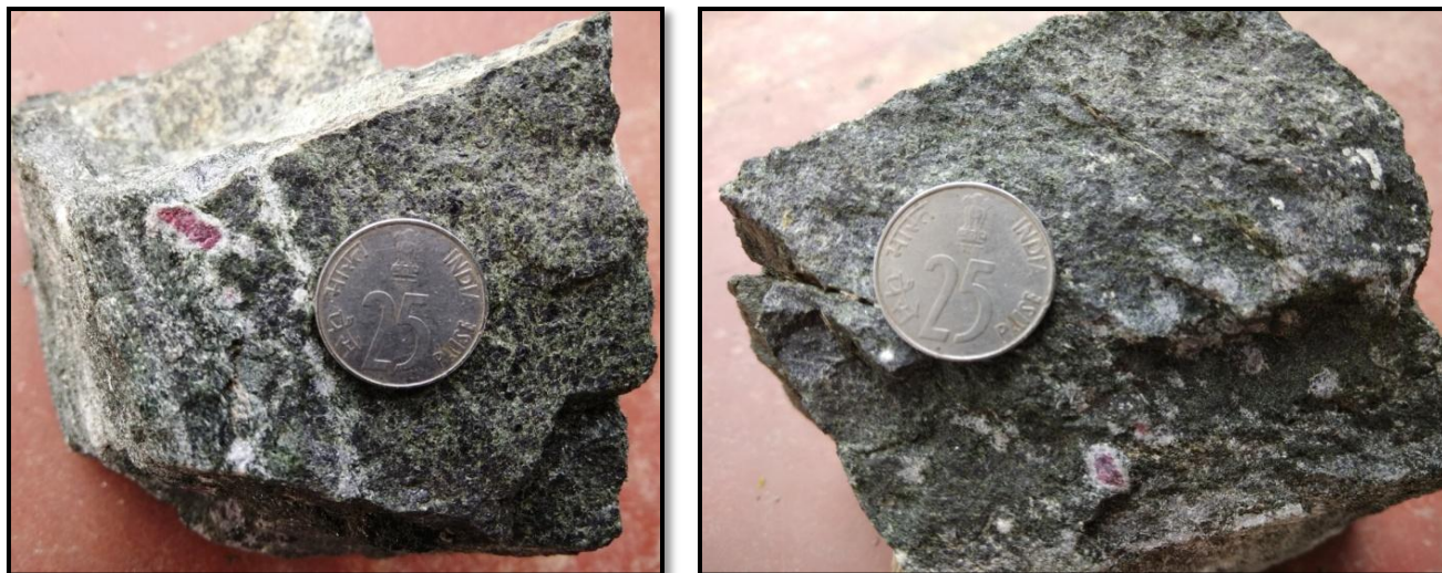
Fig.7. Hand specimen of Corundum bearing Amphibolite schist rock Collected samples Magadi area of Ramanagara district
