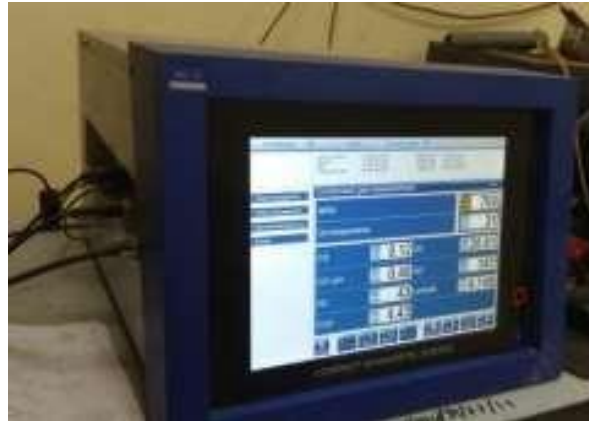
Figure 6: AVL Exhaust gas analyzer
