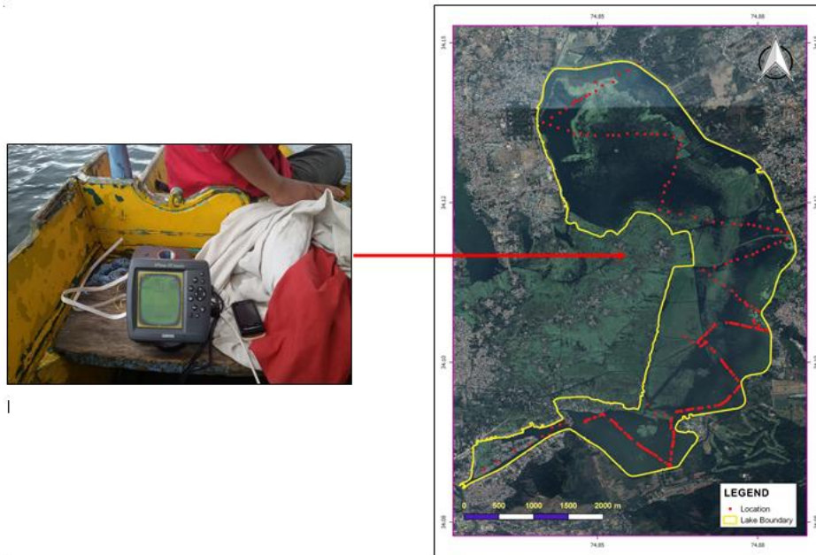
Figure 2: GPS Echo sounder setup and bathymetry collection in Lake Dal
