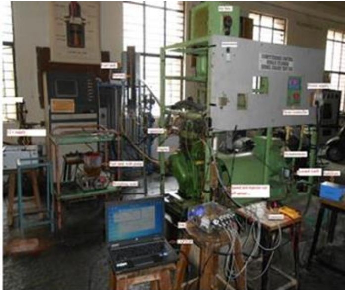
Figure 1: Experimental setup of HCCI engine testing
